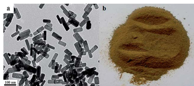
Fig. 6 (a) Typical TEM image of 25 nm × 50 nm MnWO 4 nanobars and (b) one photograph of ~16 g of 6-aminohexanoic acid-capped MnWO 4 nanobar powders synthesized using [Mn 2+ ] = [WO 4 2- ] of 0.122 M, 0.243 M of AHA, pH = 9, 180 °C for 20 h, in a 700 mL-sized autoclave.
