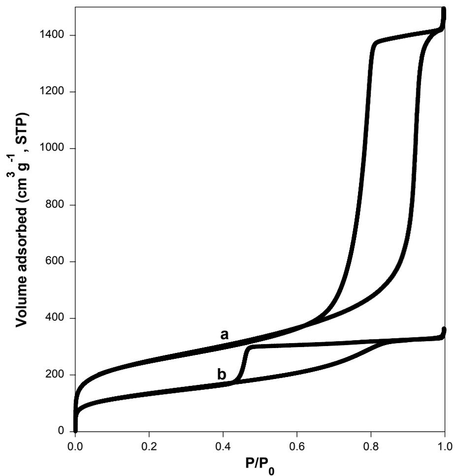
**Fig. S1:** N<sub>2</sub> adsorption/desorption isotherms at -196°C for: a) parent MCF and b) NaY coated MCF.
