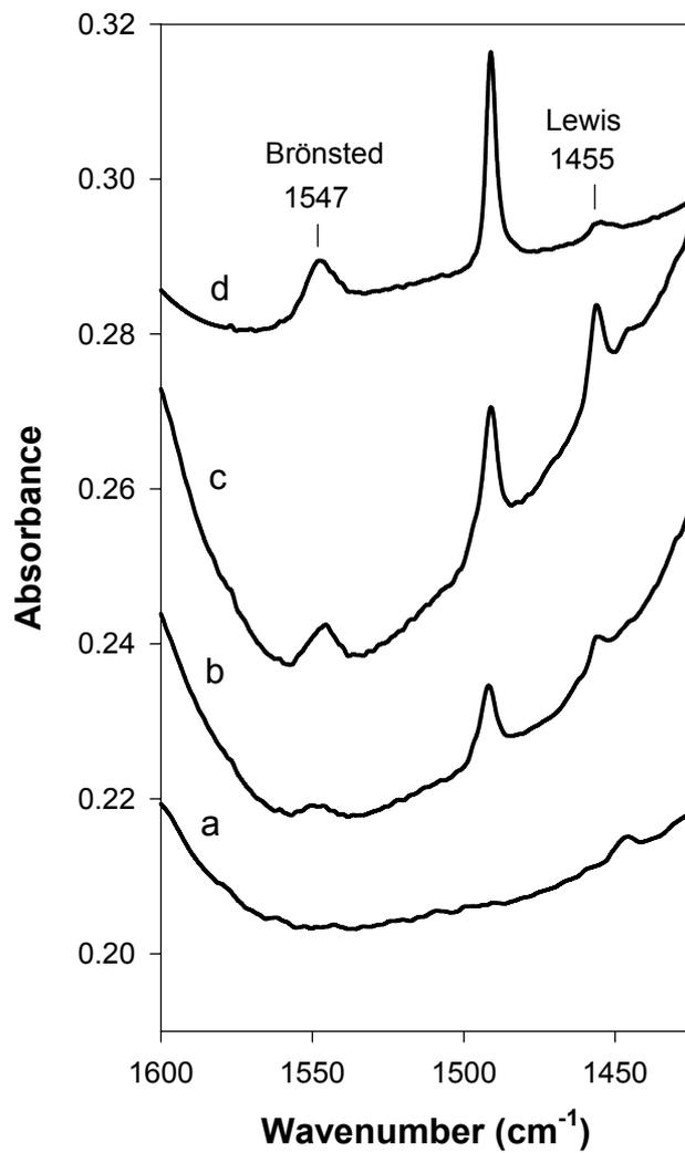
**Fig. S2:** FT-IR spectra of pyridine adsorbed on the protonated samples in the 1350-1600 cm<sup>-1</sup> range after pyridine adsorption and then desorption at 150°C: a) parent MCF in H-form, b) H-ZSM-5 coated MCF, c) HY coated MCF and d) H-ZSM-5.
