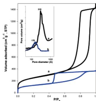
**Figure 1.** N<sub>2</sub> adsorption/desorption isotherms at –196 °C and BdB-FHH pore diameter distributions calculated from the adsorption branch of the isotherm (inset) for (a) parent MCF and (b) ZSM-coated MCF.
