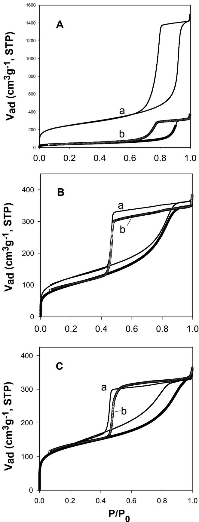
**Fig. S3:**  $N_2$  adsorption/desorption isotherms for (A) parent MCF sample, (B) ZSM-5 coated MCF and (C) NaY coated MCF a) before and b) after steaming with 20%  $H_2O$  in  $N_2$  at 800°C for 2 h.
