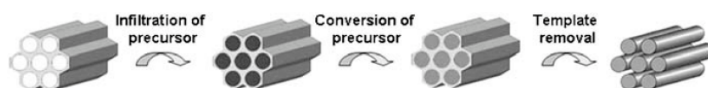
Figure 10.23 Schematic illustration of the nanocasting pathway, showing the change of the mesostructure during the process. In general, the process includes three steps: (i) precursor infiltration inside the mesochannels of the silica template; (ii) conversion of the precursor inside the nanochannels; (iii) selective removal of the mesoporous silica template [102].
