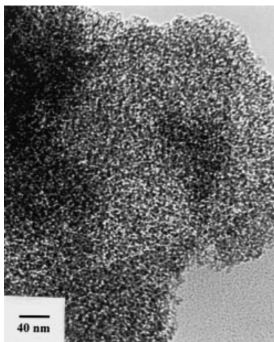
Figure 4. TEM image of the calcined [0]UL-ZSM-5 sample.
