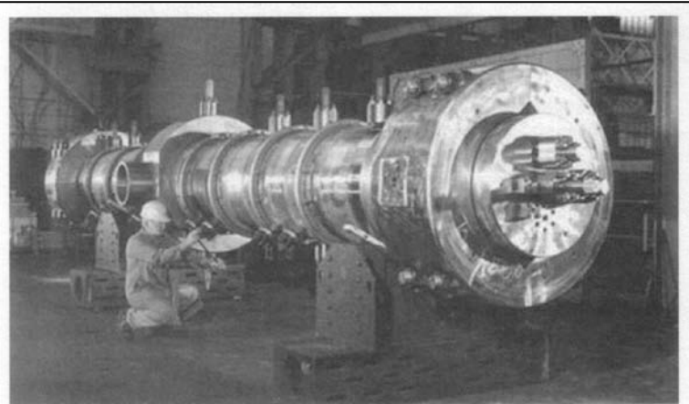
Polyethylene reactor; this 16-in inner-diameter reactor is designed to operate at 35,000 psi and 600°F; in operation, this reactor is in a vertical configuration. Courtesy of Autoclave Engineers, Division of Snap-tite, Inc.
